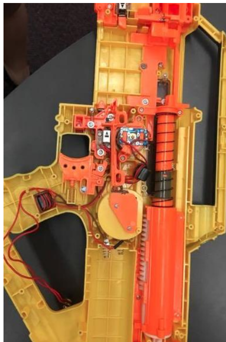
Figure 5.6: Inside of a Nerf-blaster (Team Supplied)
